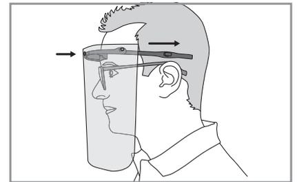
Put on the face shield by holding the temples of the visor carrier at forehead height and sliding them horizontally towards the back of the head. Spectacle wearers can also place the carrier on the frame of their glasses.
