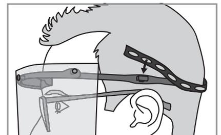
For extra stability, attach the buttonhole elastic strap to the rear mounts of the visor carrier and adjust it as required.
