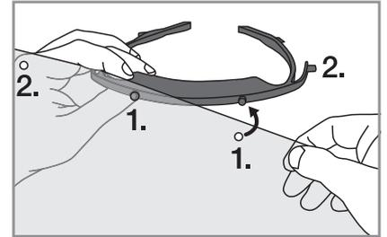
First, press the two centre holes of the foil onto the mounts on the visor carrier. Continue with the two outer holes. Your face shield is now ready for use.
